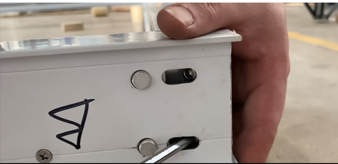
3. Tighten the screws which in holes of top and bottom frames.
