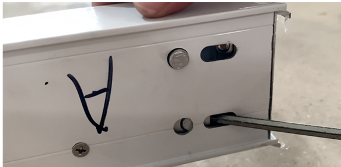
2. Pry the module spring points out of the round holes on left and right frames.
