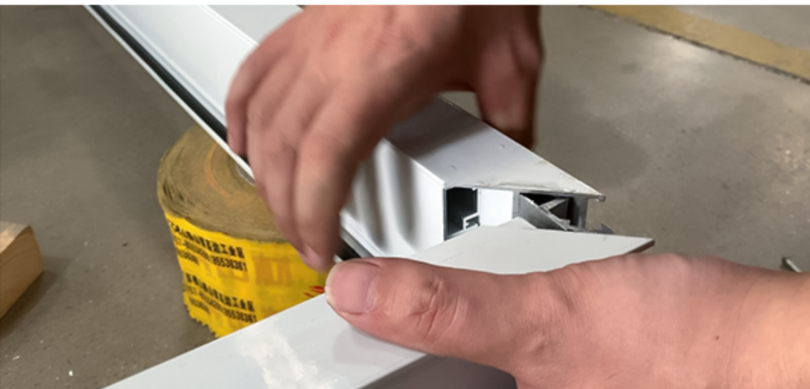
1. Insert the modules which is on the side of top and bottom frames into the 45° beveled frame.
